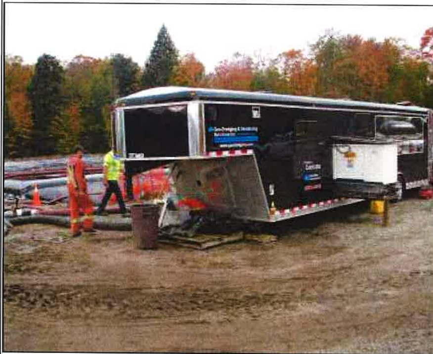
Geo-dredging and Dewatering Solutions custom designed mobile chemical conditioning system onsite at the McDougal Lagoon Project
