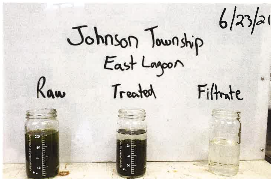
Figure 3B: East Cell showing raw sample, treated sample and RDT filtrate
