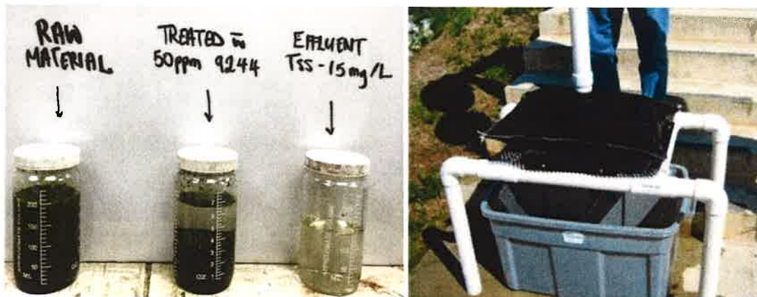
Figure 1. Routine jar testing (left), Geotube® Dewatering Test (GDT) (right).
