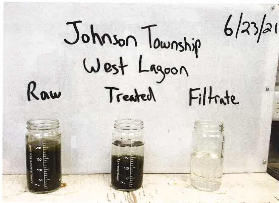
Figure 5B: West Cell showing raw sample, treated sample and RDT filtrate
